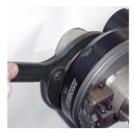
The TTSRD machines are portable and made for orbital tube cutting. These machines can be opened in two half-shells.
