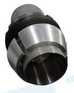
The two parts of the nut must positioned on the tube. Next the collet is positioned relative to the outside diameter of the tube. Then the machine is positioned on the tubes (see the photo enclosed).
