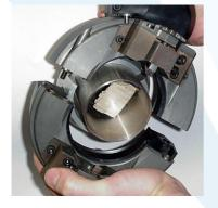
Operation 3: Clamping of the machine nut on the tube.
