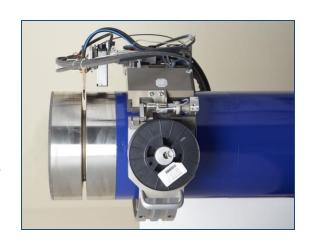
Open type carriage welding heads Polycar PLC O.D. ≥ 168 mm
