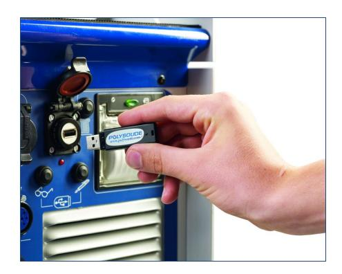
USB memory stick for saving, loading and archiving of welding programs and monitored welding data
