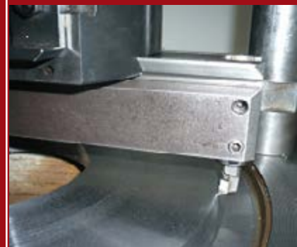
Machining RTJ groove bearing surfaces
