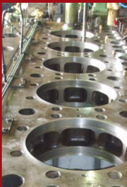
Machining 6 cylinders + positioning inserts in ten days.
