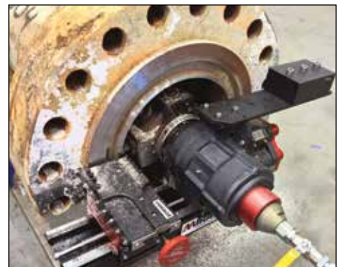
▼ MM860I machine to ensure flange joint integrity.
