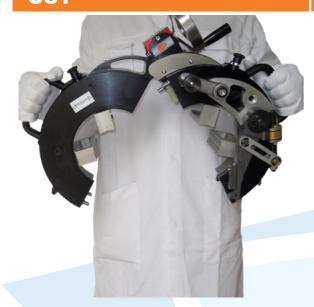
The ULTIMATE SPLIT 1 has been engineered to fit tube cutting applications in a fabrication workshop or at the job site. This wireless machine can also be bench mounted onto the ULTIMASTER Bench Unit
