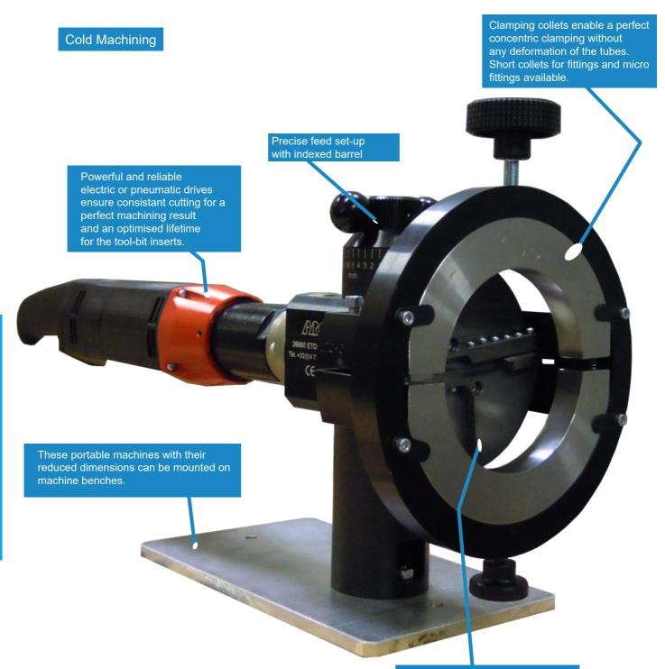
Tool-holder plates enable the facing and beveling of tubes, fittings, micro fittings and tee fittings. Machining can be performed on all types of materials (mild steels, stainless steels, alloys). Chips are contained and easily collected in order to avoid altering the integrity of the tube.
