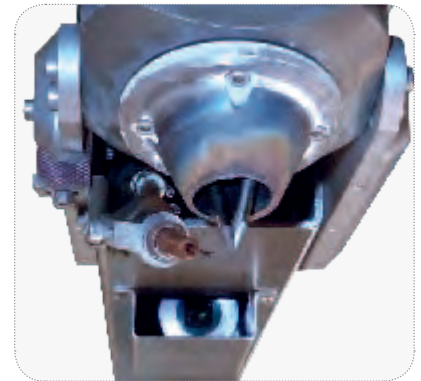
TIG er lance with integrated camera
