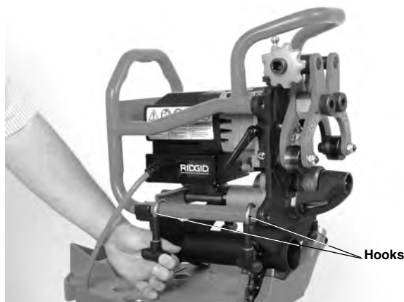
Figure 9 – Securing Beveller to Adapter
