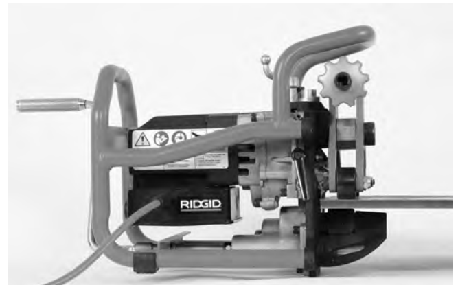
Figure 16B – Installing Beveller on Plate
