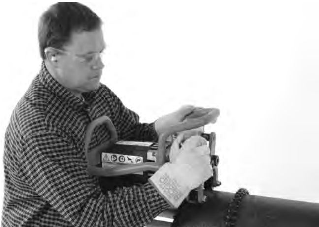
Figure 17A – Hand Tighten Clamp Screw
