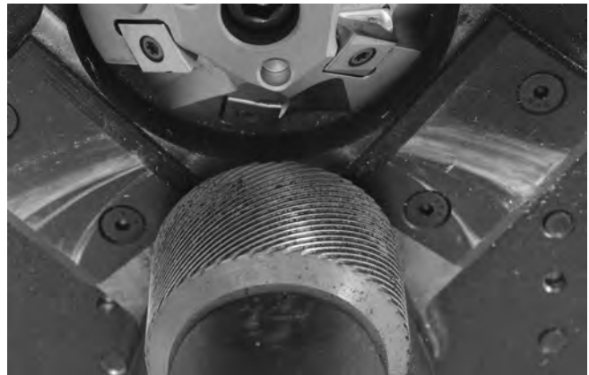
Figure 22– Clean Drive Roll Knurls
