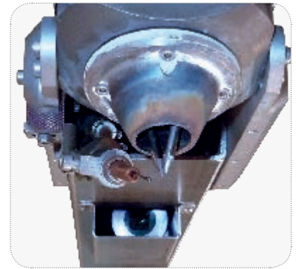
TIG er lance with integrated camera
