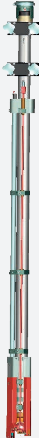
HW lance fixed angle with cameras (2C)
